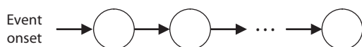
Figure 4. The tapped delay line. Several units are connected in series; activation is transmitted from one unit to the next, but with a delay. On event onset, the first unit is activated; at each time step, that activation moves forward one unit. By seeing which unit is active at a given time, one can determine the time since event onset.
